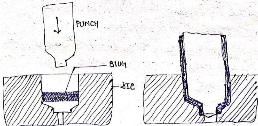
→ This process, which is shown in fig. below, the punch descends with higher velocity and strikes in the centre of the blank which is placed in die. The material deforms and fills up the annular space between the die and the punch flowing upward.
