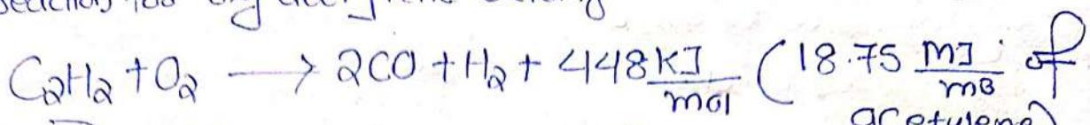
The innermost white cone temp. —  $3100^\circ\text{C}$ .
