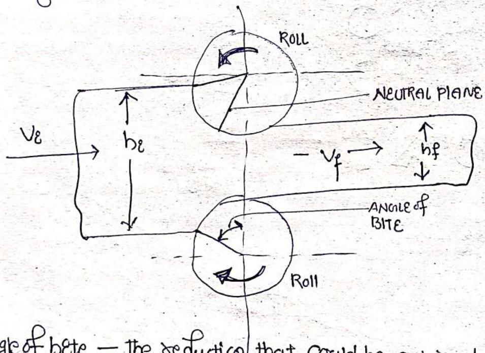
Angle of bite — the reduction that could be achieved with a given set of rolls is designated as angle of bite.
