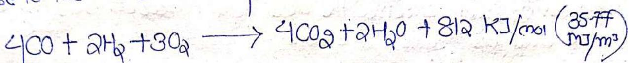
temp of bluish flame — ( $1200$  to  $2000^\circ\text{C}$ ) — Preheating steel distributed large area
