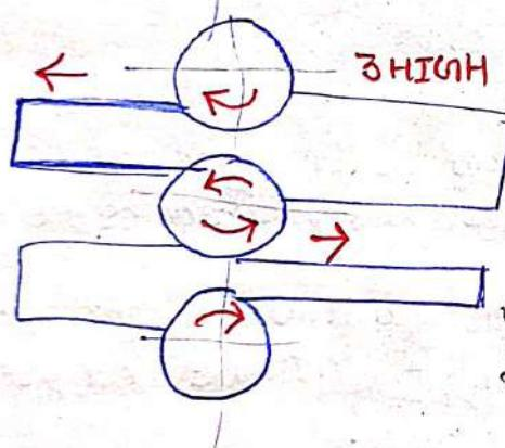
→ two continuous passes in a rolling sequence
