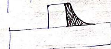
flat (flush) single V butt weld with flat (flush) backing bar
