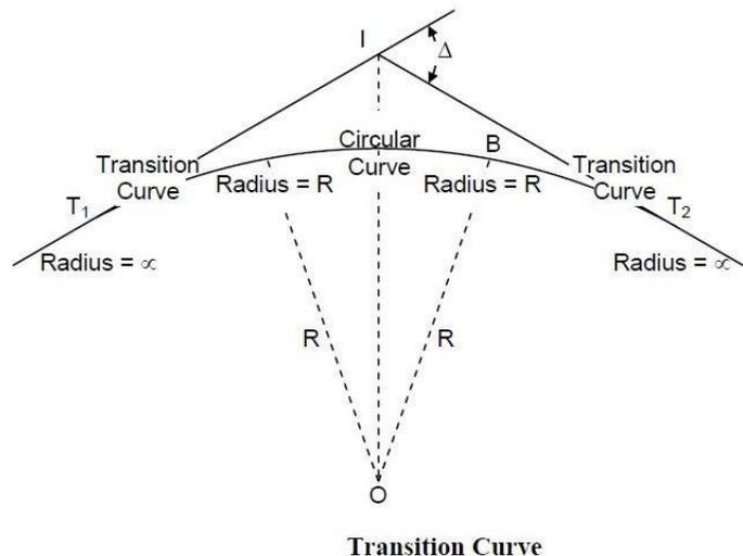
On a straight track, its two edges are at the same level. On a circular arc the outer edges are elevated depending on the radius of the curve and the speed to the vehicles expected, to avoid overturning of the vehicles due to centrifugal force acting on them while moving on circular path. Also, there is an abrupt change in direction when the alignment changes from straight to circular curve and vice-versa.
