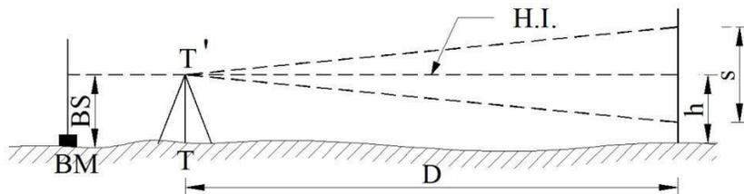
When the line of sight is horizontal, the general tacheometric equation for distance is given by
