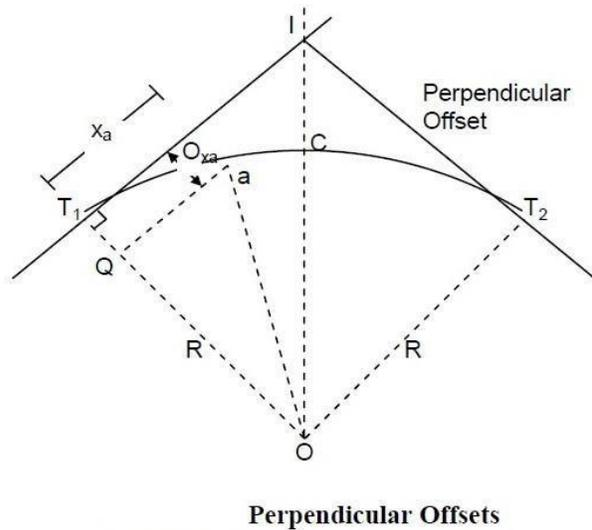
Before setting out a curve, a table of offsets for different values of  $x$  (e.g., 10m, 20m, 30m, etc.) is made. Then from  $T$  the distances  $x_1, x_2, x_3$  etc., are measured along the tangent and the
