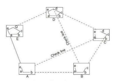
Resection Method: This method is suitable for establishing new stations at a place in order to locate missing details. It is the process of determining the previously plotted position of any peg station, by means of sight taken towards known points, the location of which has been plotted.
