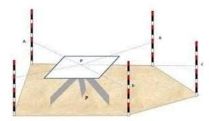
Intersection Method: In previous method it was possible to measure every distance on the field manually. In case of a mountainous terrain or rough surface where distances cannot be taken physically, it is best to use intersection method. The procedure is:
