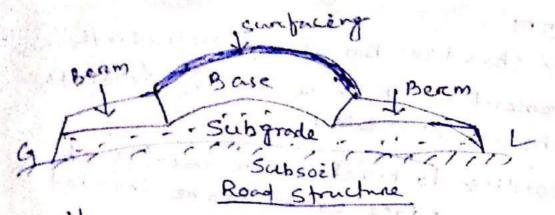
Subsoil This is the natural one prepared soil on which the repad has to be foremed . 9t should be stable and strong to carry safely the traffic load and weight of readway.
