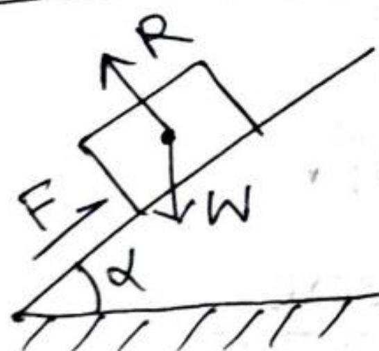
The angle of inclined plane ( $\alpha$ ) at which a body just begins to slide down the plane is called the "angle of friction".
