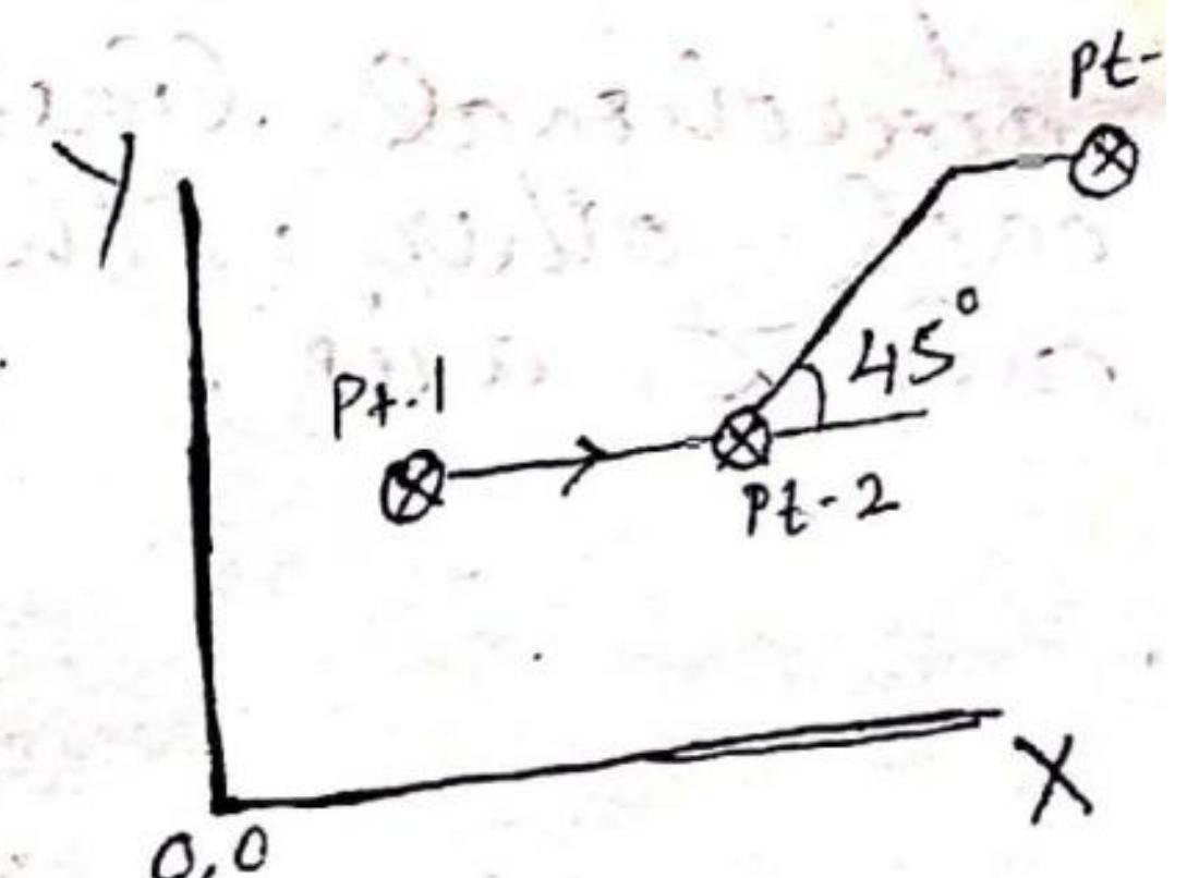
2. Straight Cut:- In straight cut moves parallel to one of the major axes at a desired rate suitable for machining. It is quite appropriate for milling workpieces of rectangular configuration. However in this process no angular cuts on the workpiece is possible. Any NC machine tool capable of straight cut movement can perform point to point operation also.
